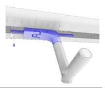
5. Remove the lower stop bolt (5mm hex key) from the right handle carriage.
