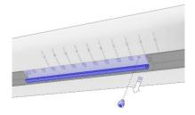
6. Lift the right handle release lever and continue to slide the handle to the top of the track. Release the lever and ensure the handle locks into place.
