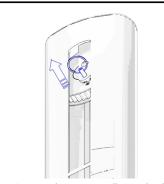
Remove pin from the upper pulley on both uprights.
