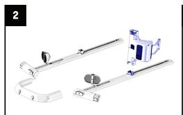
Lower console onto left upright. With upright pins still installed, the pedal or handle can be moved up and down to help align couplers.
