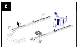
Lower console onto left upright. With upright pins still installed, the pedal or handle can be moved up and down to help align couplers.
