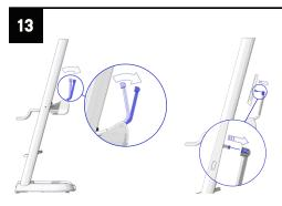
Push the display tubes back and slide the display onto the mounting bracket.
