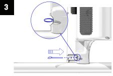
Insert Console Pin (A) into upright coupler and console. Ensure the ring on the pin sits flush in the curved surface. Rock the console to help align the holes.
